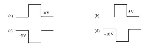
Sol: The p-n junction diode is a half wave rectifier which produces output in forward biased mode only. Thus, there will be no output corresponding to -5V input. Hence, output will be obtained corresponding to +5V only.
