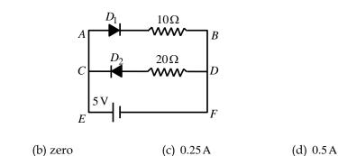
Sol: Here  $D_1$  is in forward bias and  $D_2$  is in reverse bias so,  $D_1$  will conduct and  $D_2$  will not conduct. Thus, no current with flow through DC.
