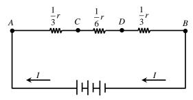
That is three resistors connected in series, between points *A* and *B*.
