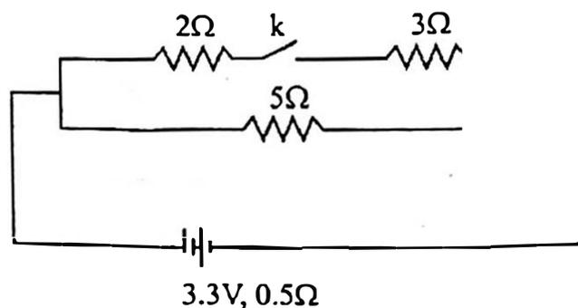
The diagram above shows a circuit with the key k open. Calculate:
