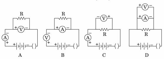
Which one of the following is the correct set-up for studying the dependence of the current on the potential difference across a resistor and why?
