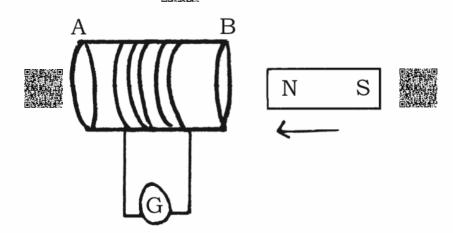
What type of current is induced in the coil by doing the experiment related
