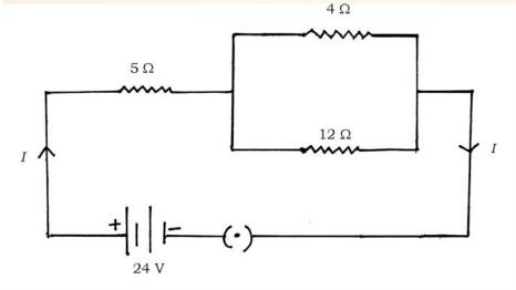
Calculate the total resistance and the total current flowing through the circuit.
