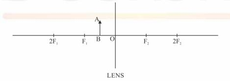
Copy the diagram and by using three standard rays starting from point A, obtain an image of the object AB.
