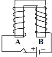
The diagram shows a coil wound around a U shape soft iron bar AB.
