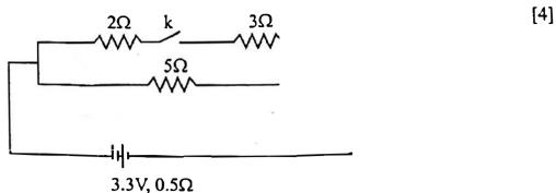
The diagram above shows a circuit with the key k open. Calculate:
