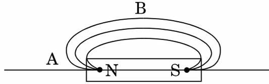
Magnetic field lines are shown in the given diagram. A student makes a statement that the magnetic field at 'A' is stronger than at 'B'. Justify this statement. Also redraw the diagram and mark the direction of magnetic field lines.
