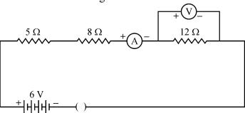
What would be the readings of the ammeter and the voltmeter when key is closed? Give reason to justify your answers.
